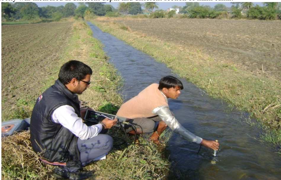
Plate 2.2 : Measurement of canal water flow velocity in head reach
